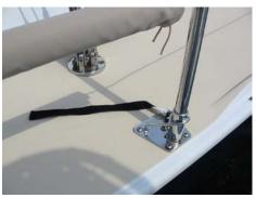
This is one of two methods used to secure the spinnaker halyard to the rail. This boat was using Velcro to hold the halyard.
