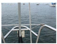
Simple shock cord used to keep the tack higher when the A-sail is being pulled out on the set. This helps prevent the heavy tack material from getting wedged between the sail and the bow pulpit, as well as the jib from catching the rail when unfurled.
