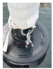
Wichard Snap Shackles were seen on 90% of the boats for the tack of the jib and the head of the jib to prevent the bowman from losing the shackles when removing the sail after racing.
