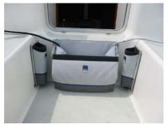
Blue Performance line bag and winch handle holders. The nice thing about these is that they weather better and can be removed easily for winter storage. This boat has the large bag and we have found that the Medium bag works best is this location so that the winch holders can also mount to the front face of the cockpit.
