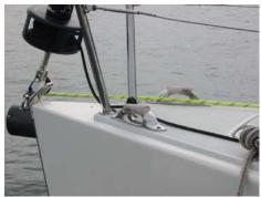
Reinforced vinyl tubing used on chocks to prevent lines from catching.
