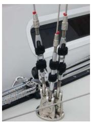
APS and Team One sell these shroud pin systems that allow easy access to tuning the rig. Each Velcro strap has a short cotter pin and the Velcro keeps it in place and protects from any sharp edges. This is a much better idea than tape and bending split pins each time you want to adjust the rig.
